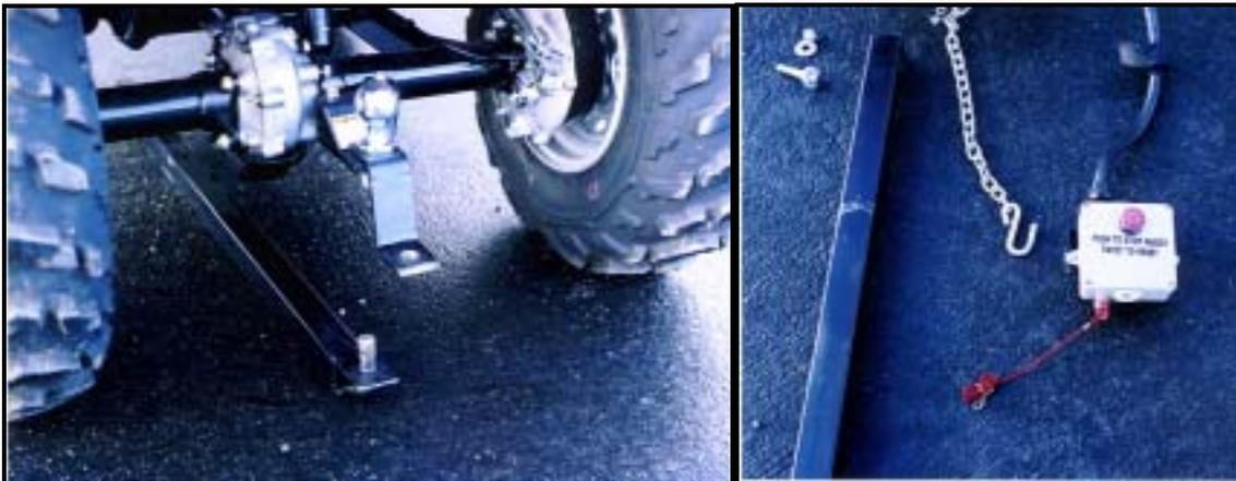
In order to keep you safe when operating the **SnowHogg**, we made the control box adjustable, so it can be mounted within reach on the front rack of your
